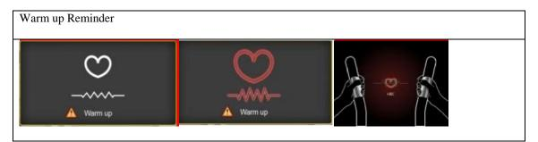
When exercise start, there is 2 minutes Warm up time. If no hand pulse input, system will alarm and remind user to grip handlebar. Without pulse input for 30 seconds, console will stop.
