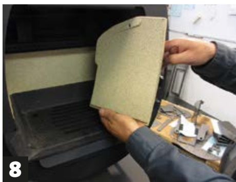
8 Mount the right side plate in the same way as the left plate
