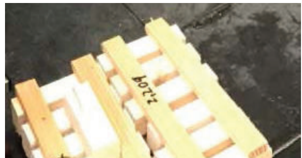
Placement of the fuel load in the firebox
