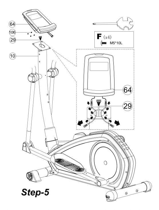
Assemble the upper computer cable (29) to the computer (64). Through the handle pulse cable attached to the computer out of the holes on the handlebar post like fig shown.
