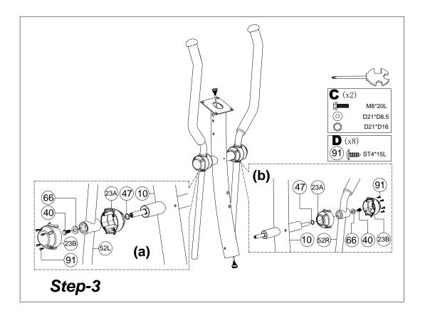
Assemble the left and right moveable handlebar (52L&52R) to handlebar post (10) by left & right upper foot cover (23a&23b), waved washer (47), flat washer (66), bolt (40) and screw (91) like picture a and b shown.
