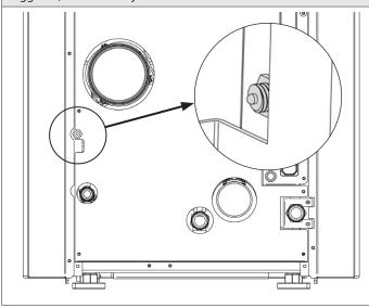
If the stove is not powered, it is recommended to have the fuse checked by a qualified technician
